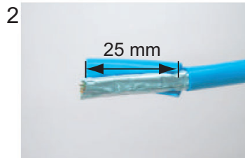
Remove the inner vinyl sheath by approx 25 mm. Be careful not to damage inner shield and cores.
