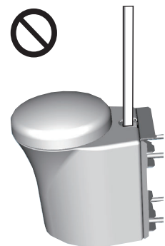
NG: Taped part can not be seen.
