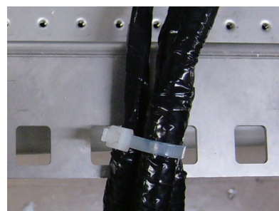
Fix cables to post with cable tie
