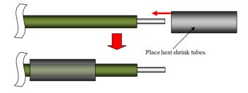
**Step 3** Move the heat shrink tubes to the soldered correction, and then apply heat to the tubes.
