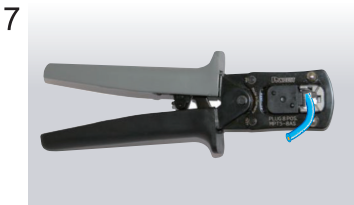
Using special crimping tool MPT5-8AS (PANDUIT CORP.), crimp the modular plug. Finally, check the plug visually.
