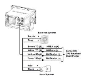
The NMEA 0183 wire should be connected to a compatible NEMA 0183 device as shown in the table below:
