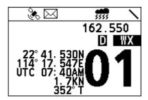
In weather mode, you can rotate the Menu/DSC to select a NOAA channel to monitor. What you selected would be mark as last used weather channel.
