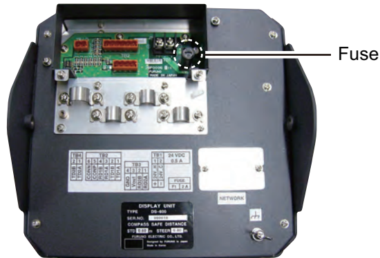
Fuse location (Rear panel: cable cover removed)
