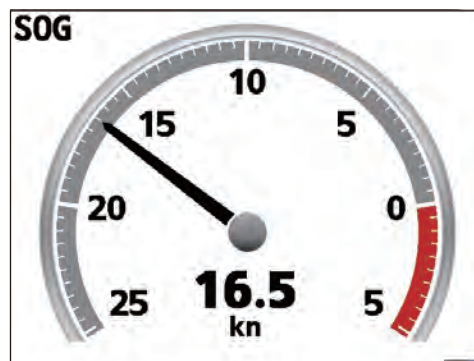
Symbol Location: Right (The pointer rotates counterclockwise as ship's speed increases.)
