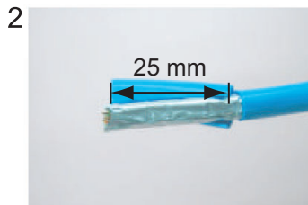
Remove the inner vinyl sheath by approx. 25 mm. Be careful not to damage inner shield and cores.
