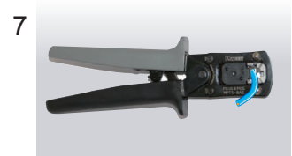
7 Using special crimping tool MPT5-8AS (PANDUIT CORP.), crimp the modular plug. Finally check the plug visually.
