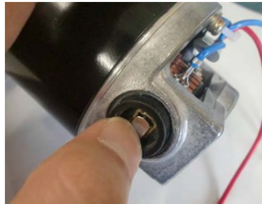
Depress the carbon brush into the holder.
