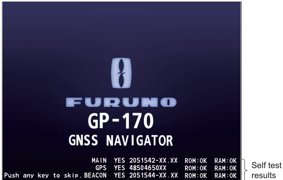
Self-test display at equipment start up
